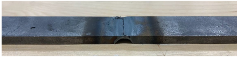
Figure 66: Bottom View Image of Robot Weld
